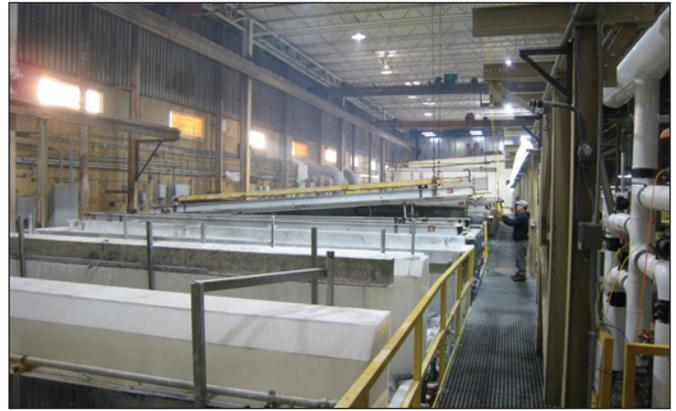
A new anodizing line at Futura provides automated process controls and has increased capacity by 30%.
